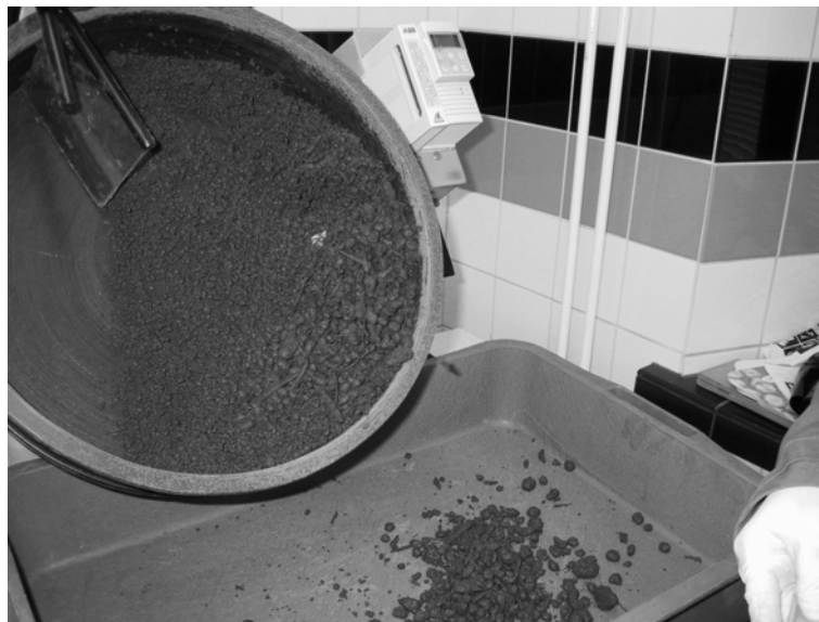
Figure 1. Laboratory disc pelletizer, diameter 0.4 m [10].
